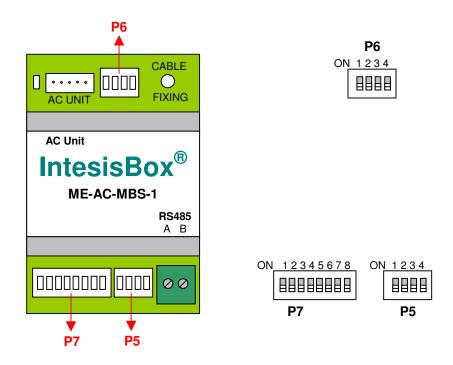
The following table applies for configuration of the interface through these DIP-switches:
